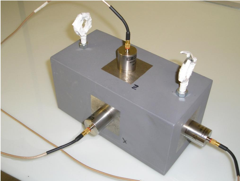
**Figure 2:** 35 lb. steel block with three mounted accelerometers.
