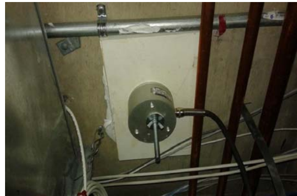
Figure 5 Interior measurement setup adjacent to an operating room, ceiling plenum equipment shelf (left) and under slab accelerometer mounting (right).
