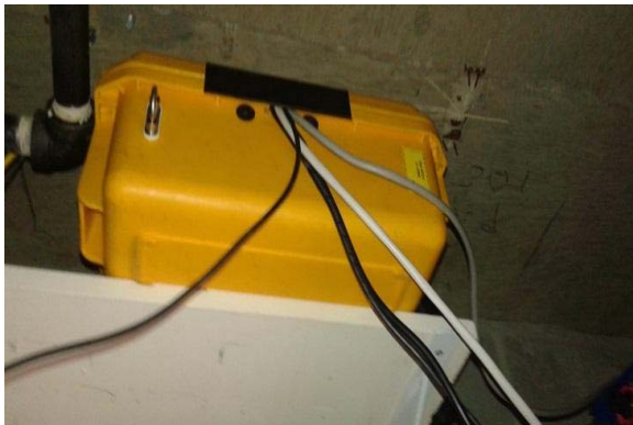
Figure 5 Interior measurement setup adjacent to an operating room, ceiling plenum equipment shelf (left) and under slab accelerometer mounting (right).
