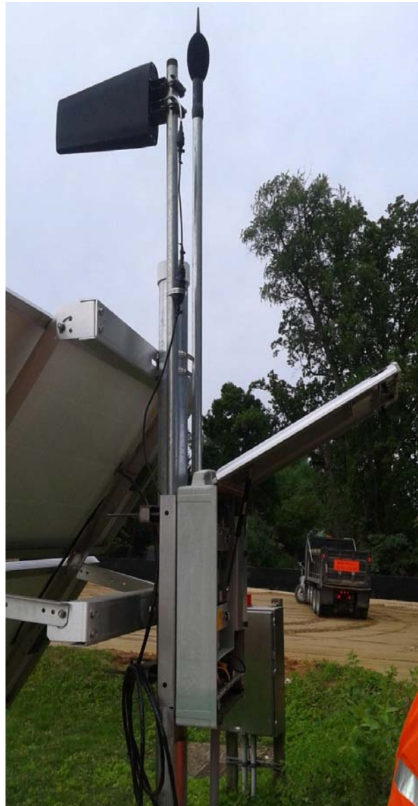
Figure 1 Instrument Setup on Pole. Note microphone & cellular antennae.
